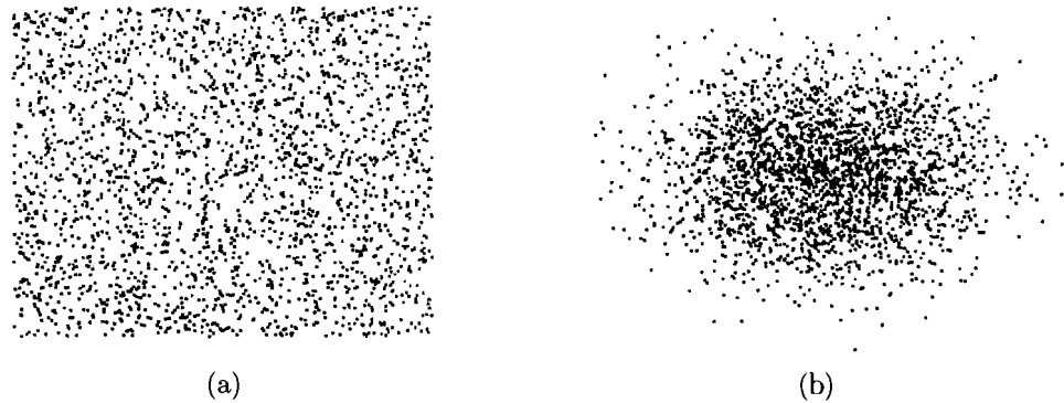
Figure 1.9: Comparison of uniform samples in the C-space with corresponding samples in the task space. (a) 1000 samples evenly in the C-Space. (b) Corresponding end-effector positions in the task space computed from forward kinematics equations.
