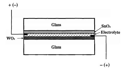
Figure 2.3 Experimental arrangment for coloring and bleaching WO<sub>3</sub> films deposited onto both glass and SnO<sub>2</sub>:F substrates
