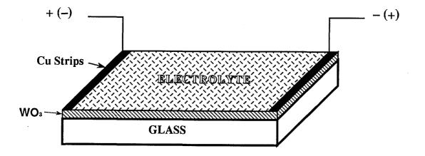
Figure 2.2 Experimental arrangment for coloring WO3 films deposited onto glass slide
