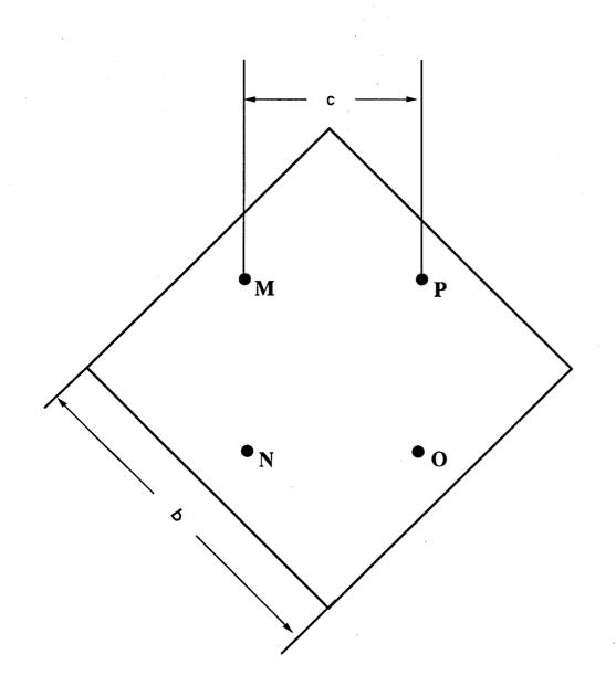
Figure 2.4 The diagram for Hall measurements showing a separating spacing of four-point contacts c=13.68 mm, and the length of squares sample b=25.45 mm
