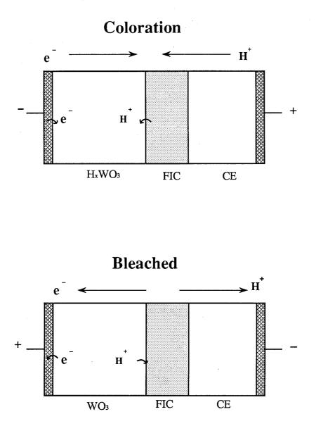
FIC: Fast Ion Conductor CE: Counter Electrode
