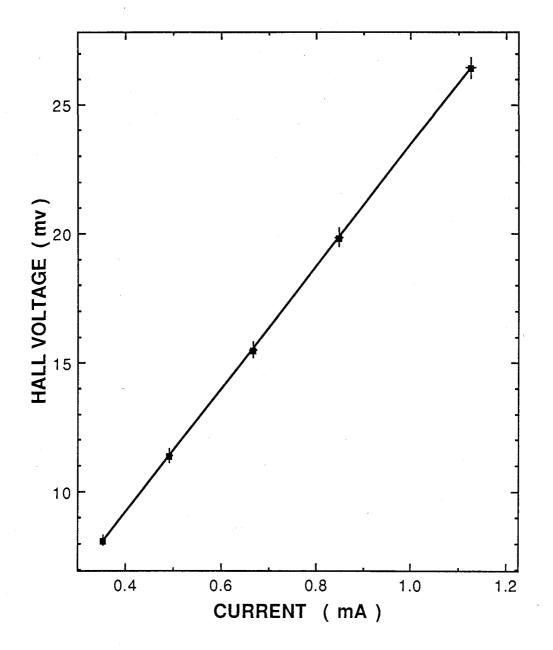
Figure 2.6 The relationship between the applied current  $I_{Mo}$ and the Hall voltage V while keeping B constant for WO3 film prepared on glass at substrate temperature 350°C
