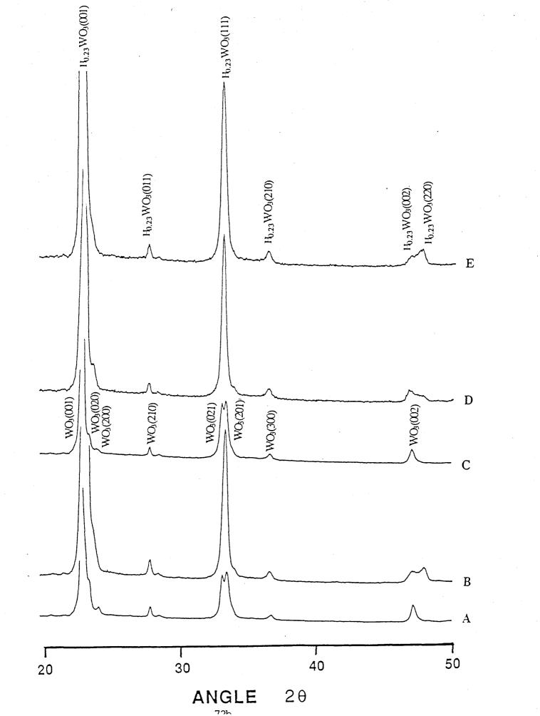
Figure 3.11 X-ray diffraction patterns showing the structural changes during the electrochromic process in WO3 film prepared on SnO2:F substrate at 400°C for
