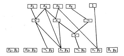
This Boolean circuit has 8 sources, 6 input gates, and 7 sinks or output gates. Its size is 16, its depth is 3, and it has fan-in 3.
