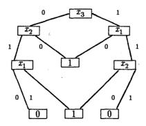
This branching program is levelled, has size 9, length 3, width 3, and computes the
