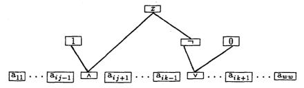
C is a fan-in 2 Boolean circuit of size  $w^2+4$  and depth 2. On input 1, C outputs  $C(1)=a_{11}\cdots a_{ij-1}1a_{ij+1}\cdots a_{ik-1}0a_{ik+1}\cdots a_{ww}=\overline{f}$ , and on input 0, C outputs  $C(0)=a_{11}\cdots a_{ij-1}0a_{ij+1}\cdots a_{ik-1}1a_{ik+1}\cdots a_{ww}=\overline{g}$ .  $\square$
