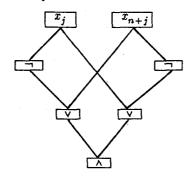
Clearly,  $C_j$  is the Boolean circuit which corresponds to the Boolean formula  $\beta_j(x_j, x_{n+j})$ . Let A be the Boolean circuit  $C_j$  excluding input gates, and let C be the Boolean circuit below.
