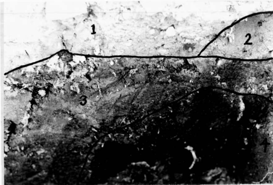
Fig. 10 Section through substrates showing margins of substrate types 1. Stony material 2. Grey silts 3. Grey silts intermingled with organic matter 4. Organic matter Section approximately 2 feet by 1½ feet
