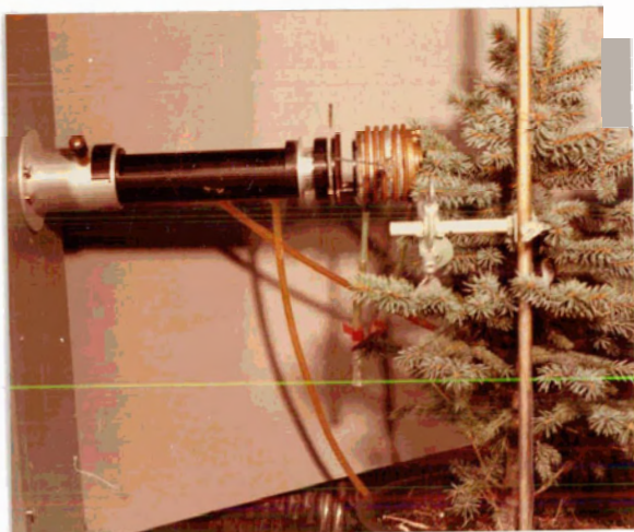
Plate 7. Complete cuvette and light-train assembly in operating position.
