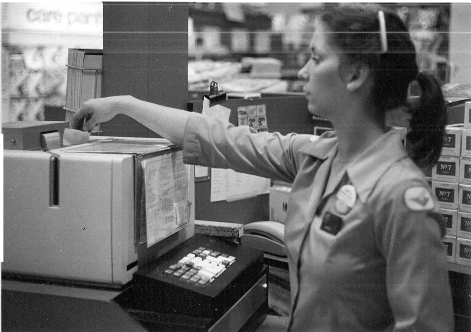
Excessively high placement of the receipt-giver, necessitates repetitive lifting of the arm.
