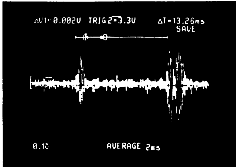
Figure 5.10 Return Signal of Pilings.
