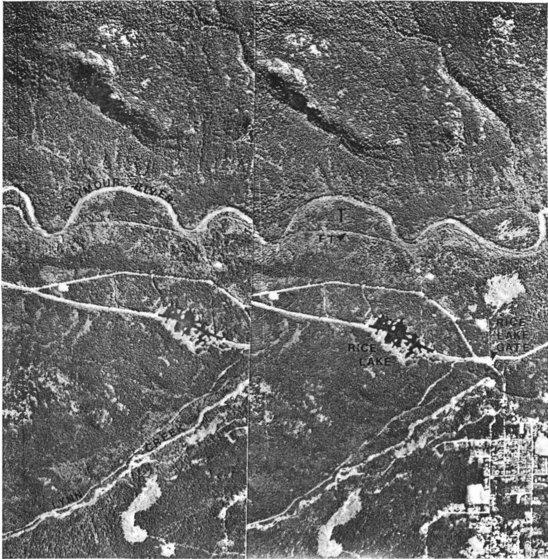
Figure 1.4 Stereopair (1:29 434) showing the valley fill near Rice Lake. FT = Fisherman's Trail; T = terrace where Unit 14 sediments are observed to overlay Unit 1 sediments (see Chapter 4).
