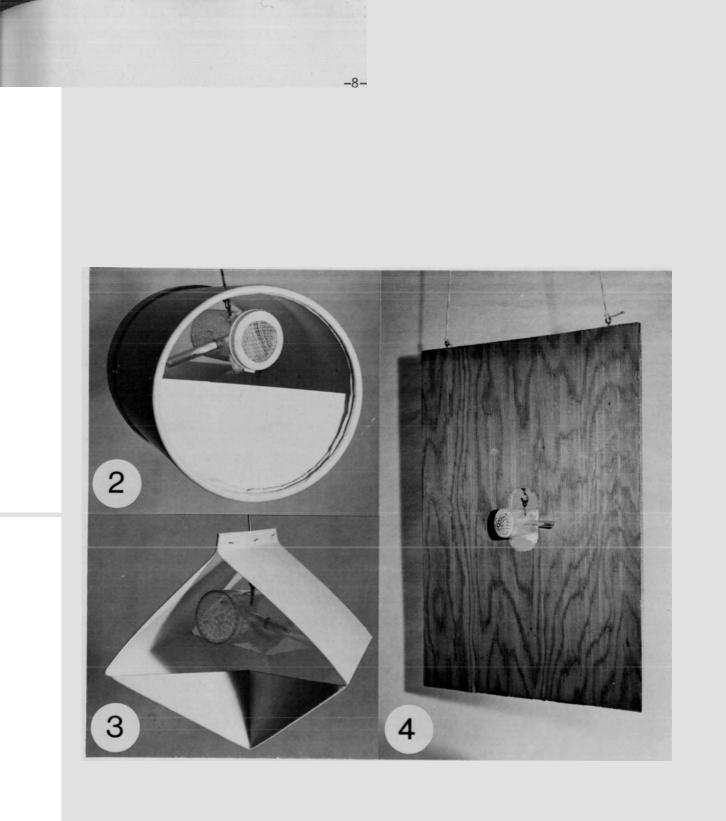
of an enlarged replica of the commercially produced 3M sectar  $\operatorname{trap}^3$ (Fig. 3). The inner, sticky surface area was slightly less than that of the cylindrical cardboard food carton. The fourth set of traps consisted of 3/8" plywood boards 30 x 43 cm with a 7.5 x 4 cm window in the centre in which the source chamber was suspended (Fig. 4). Both surfaces of the board were coated with Stickem Special.
