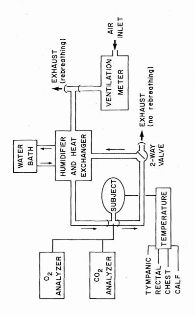
Respiratory gases were measured by continuous sampling directly at the mouthpiece. Inspired and expired alveolar carbon dioxide fractions were analyzed by a rapid response infrared carbon dioxide analyser (Godart Statham). Corresponding oxygen fractions were analysed by a rapid response zirconium oxide oxygen analyser (Applied Electrochemistry S-3A).
