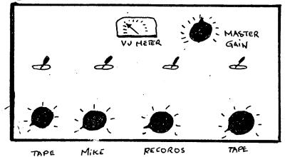
The mixer unit determined what kind of sound effect you will get. Each output has it's own volume. Adjusting these controls will give you the right balance of sound. You adjust the controls with a "pot", a large knob which registers the amount of sound output from any source.
