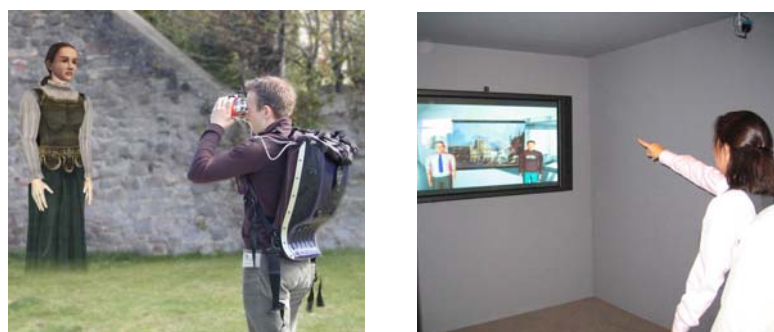
Figure 2: Special interfaces to interact with a story. Left: Geist – in the Mobile-AR scenario, interaction occurs through finding ghosts by walking in real locations. Right: art-E-fact – pointing gestures specify regions in a painting to discuss.
