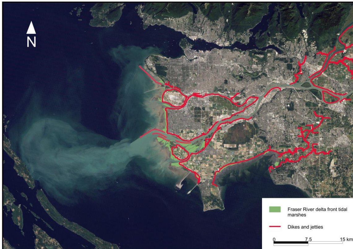
Figure 8: Extent of dikes and jetties in the Fraser River Delta in 2020. Satellite Imagery provided by NASA Earth Observatory (2011) clearly displaying sediment plume discharge from the Main Arm of the Fraser River.
