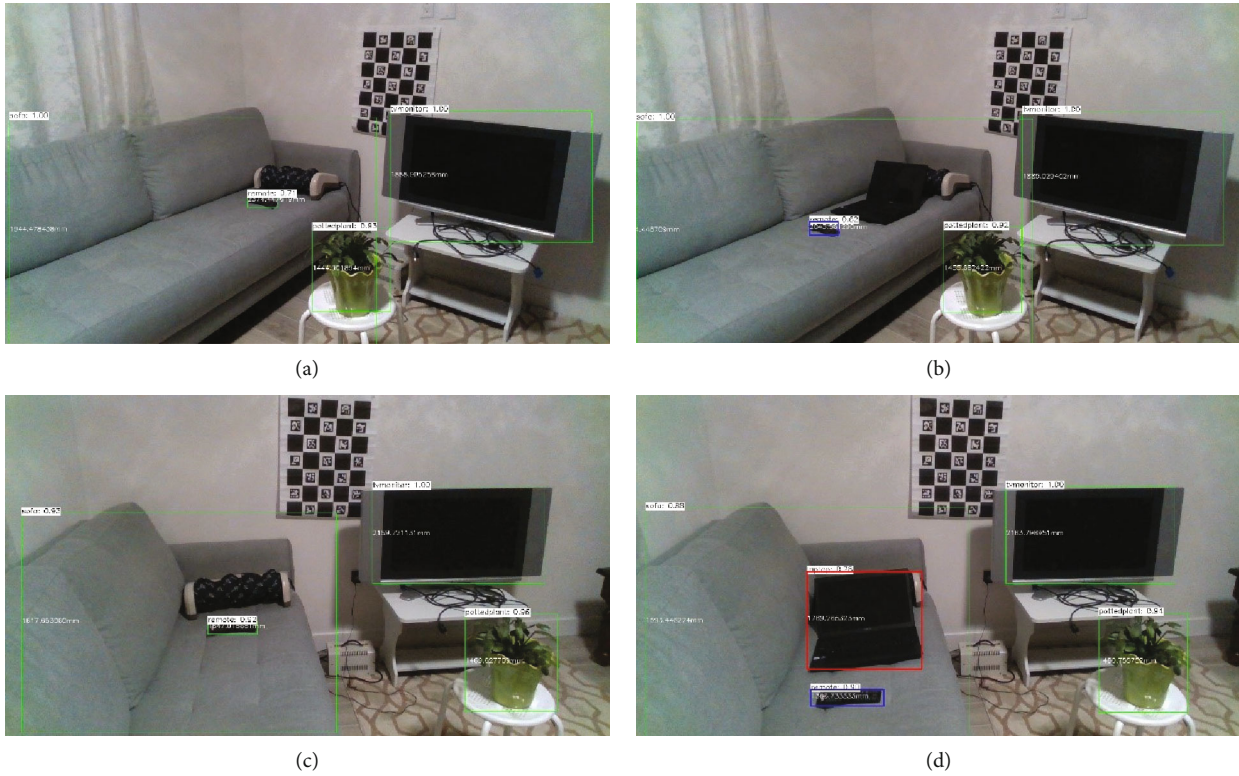
FIGURE 7: Object detection for before and after the instances when an older adult walks into the monitoring area. Left column (a, c) shows the detected objects at the initial event from left and right sensors, and the right column (b, d) shows the detected objects after the movement event.
