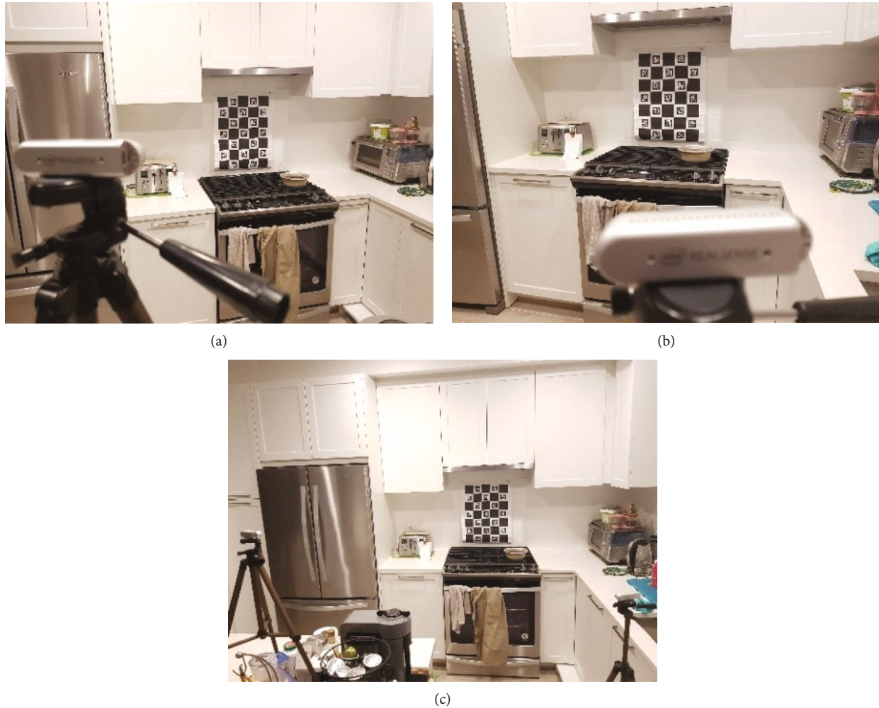
FIGURE 10: Example of sensor setup for the fourth case study including an oven, a cooking bowl, a toaster, and a microwave oven. (a, b) show views including the left and right sensors. (c) shows the full view of the monitoring area including the locations of the left and right sensor.
