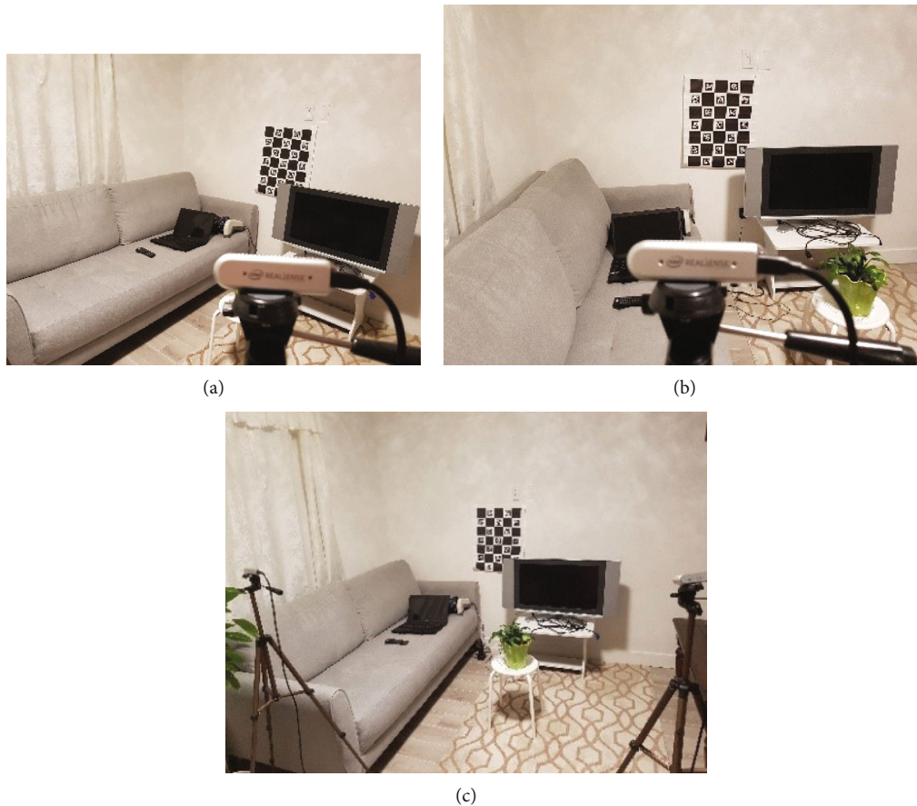
FIGURE 5: Example of sensor setup for the first case study after the older adult has left the monitoring area. (a, b) show the RGB view from the left and right sensors. (c) shows the full view of the monitoring area including the locations of the left and right sensors.
