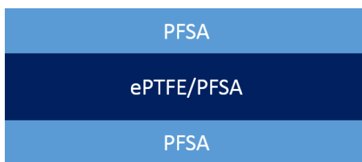
Figure 4: Schematic of ePTFE reinforced membrane.
