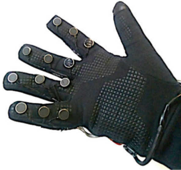
Figure 5: Singhal et al.'s Flex-N-Feel gloves for communicating touch.
