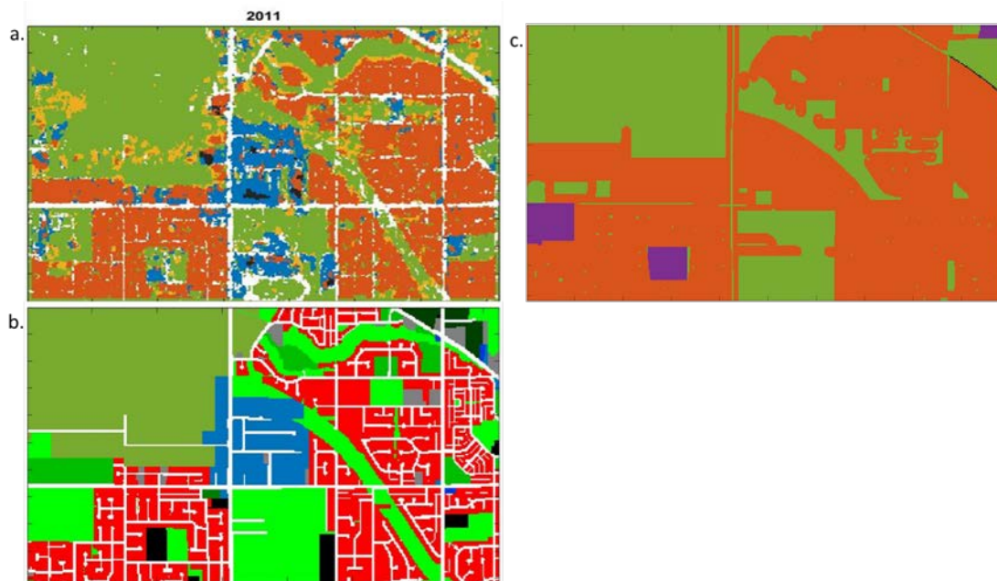
Figure 2-10 Comparison of the LU classifications for the year 2011: (a) resulting from the proposed CNN approach for the LU classification; (b) from Metro Vancouver Open Data Catalogue and (c) from DMTI Spatial Inc
