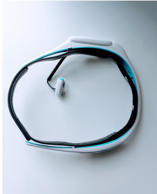
Figure 1. Photo of BrainLink Pro portable EEG headset by NeuroSky.
