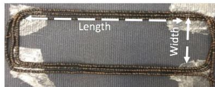
Figure 4.3 A fabricated 3-loop sensor sample.
