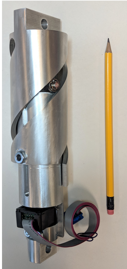
Figure 3.7: Cylindrical cam damper, manufactured
