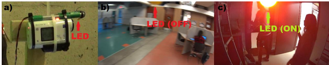
Figure 6.1. Sony ActionCam setup, wherein a) a L.E.D. is mounted on top of camera for synchronization; b) the L.E.D. is slightly seen on top portion of video frame; and c) the L.E.D. is blinked to mark an event
