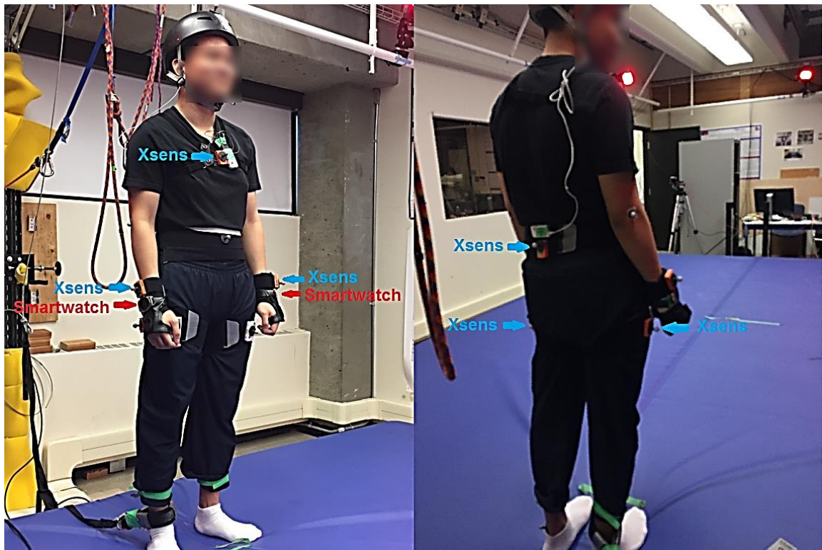
Figure 3.2. Participant standing on mattress and equipped with smartwatch, Xsens sensors, and optical motion capture camera markers
