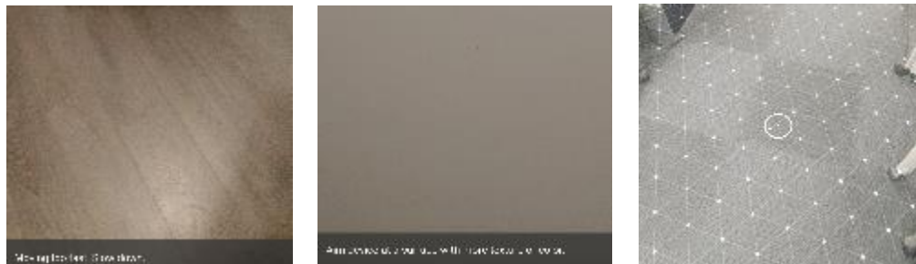
Figure 4.12 (a) Give message if device is moving too fast. (b) Provide feedback if surface is not trackable (c) draw mesh to provide feedback that ground plane is detected.
