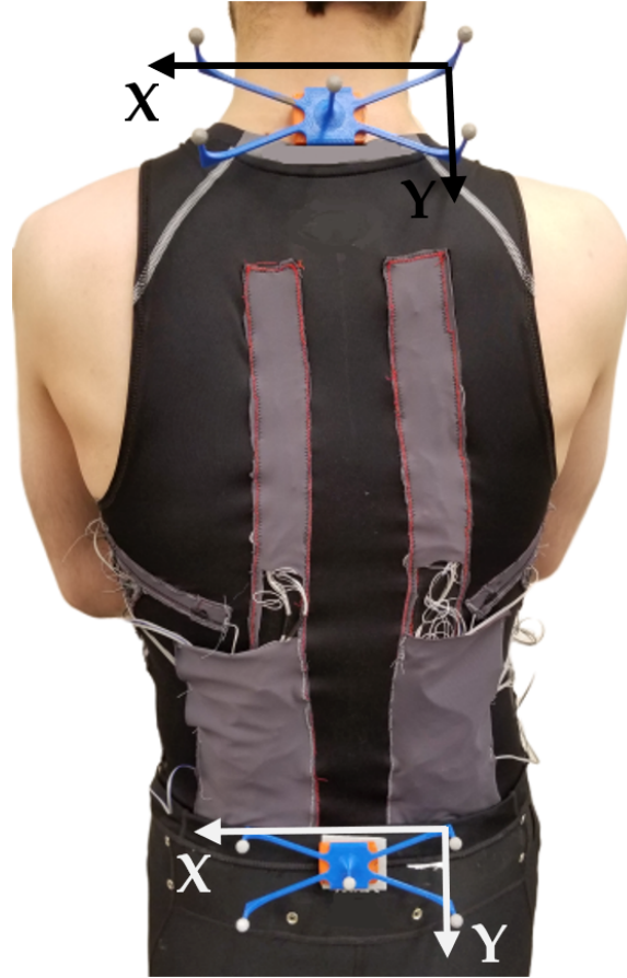
Figure 4.2: The experimental setup used for collecting trunk motion data from IMU units and smart garment with integrated fiber strain sensors.
