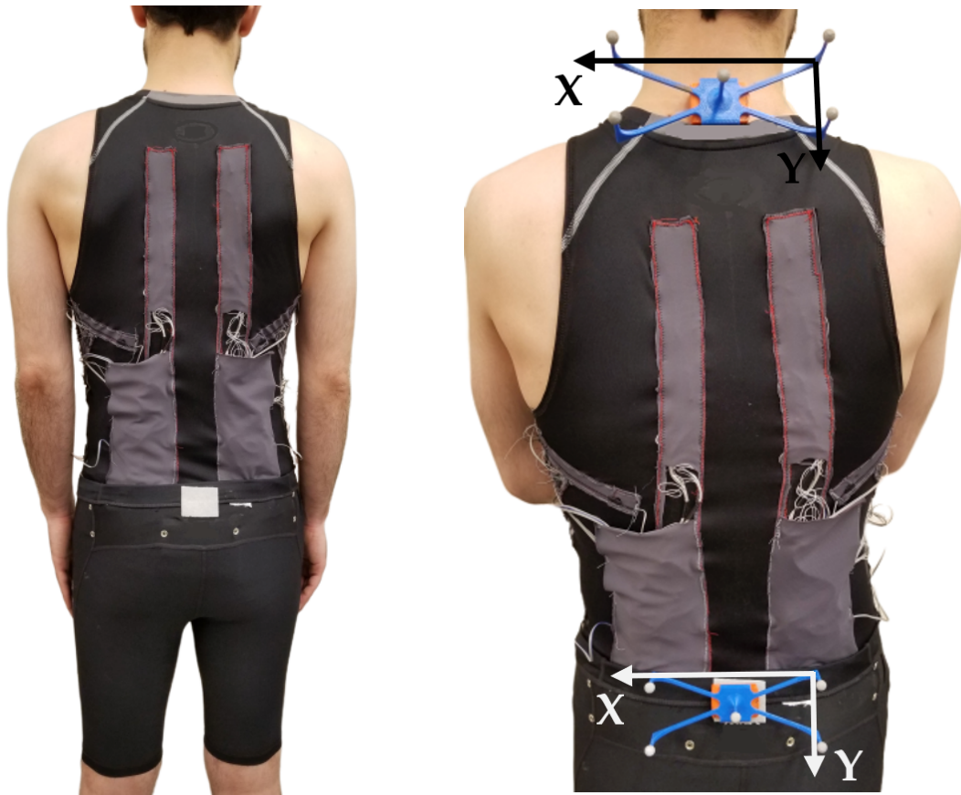
Figure 3.3: The two-piece smart prototype with sensor integrated sleeveless shirt and shorts. Sensors were integrated on the back side of the shirt into the textile. (a) A participant wearing the prototype. Shirt was anchored to shorts with Velcro patches to minimize the upward shift at the waistline; (b) Two reflective marker sets attached to participant C7 and S1 vertebrae for generating reference kinematic angles using motion capture system.
