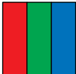
Figure 9.1 An LCD colour pixel is spatially multiplexed into three subpixels. At a suitable viewing distance, light from the subpixels is summed by the viewer's visual system.
