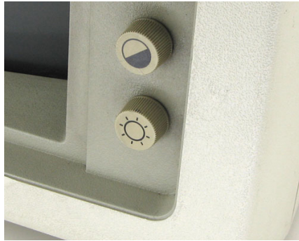
Figure 6.4 IBM 5151 PC display was introduced in 1984 with no external control names; instead, the controls were marked with graphic symbols. The symbols were subsequently standardized by IEC and ISO.
