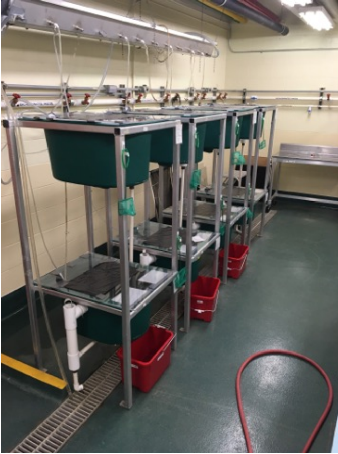
Figure A1. Shows the tank flow-through set up containing 252 juvenile rainbow trout ( Oncorhynchus mykiss ). Tank 1 was the control (n = 36) that did not receive test or reference chemicals; tank 2 was the reference (n = 36) that only received reference chemicals; tanks 3-8 (n = 36 tank -1 ) contained test fish ranging in three concentrations of octamethylcyclotetrasiloxane (D4) and three concentrations of decamethylcyclopentasiloxane (D5). It should be noted that the fish from tanks in low and medium concentrations of D4 and D5-spiked feed were extracted but are not discussed in the current study because concentrations were below the limit of detection.
