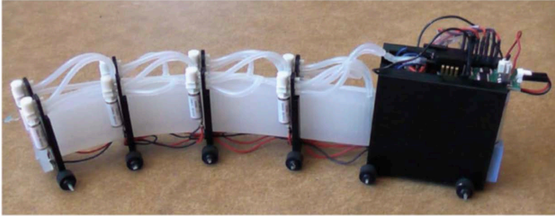
Figure 40 A soft robotic system used to mimic snake like locomotion for environmental monitoring purposes. The robot is currently limited by its bulky rigid pneumatic compressor. Reproduced with permissions from [147]
