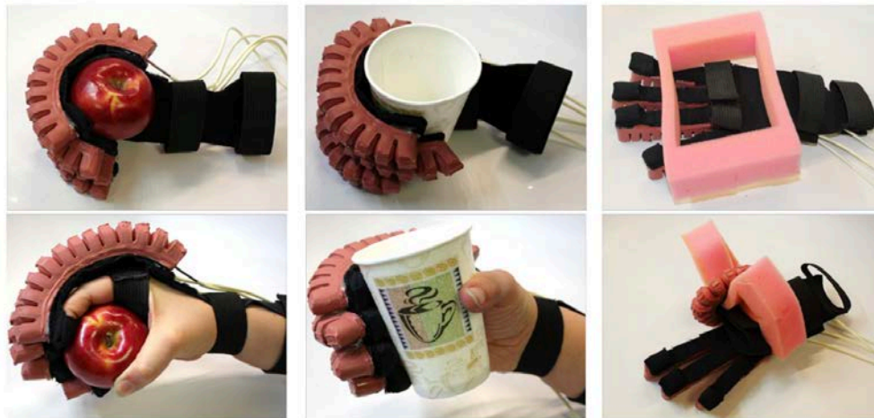
Figure 37 A soft wearable assistive device for the hand, powered by pneumatic actuators and tethered to a pneumatic compressor. Reproduced with permissions from [145]
