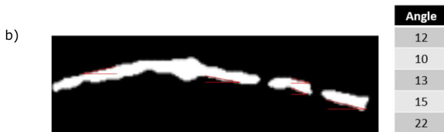
Figure 4.8: a) Plot for the effect of catalyst layer undulation angle on average value of catalyst layer thickness and approximate acceptable error; b) Measurements of catalyst layer angles for a highly undulated region, with measured angles shown.
