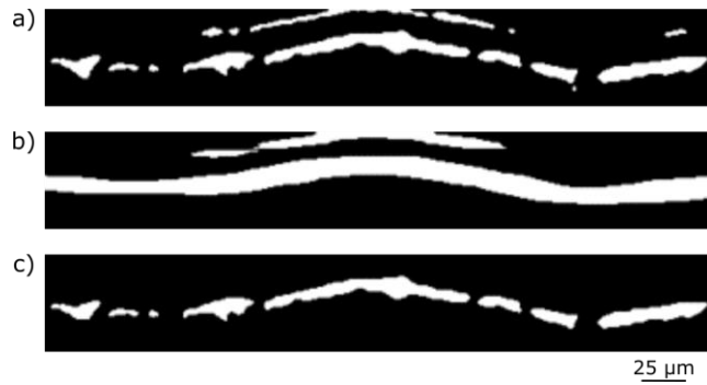
Figure 4.6: a) Initial segmentation following crop and thresholding from in-situ XCT image. b) 2-dimensional Gaussian blur applied and thresholded to connect cathode as single object. c) Using binary logic to select only the cathode catalyst layer from volume selection of b).
