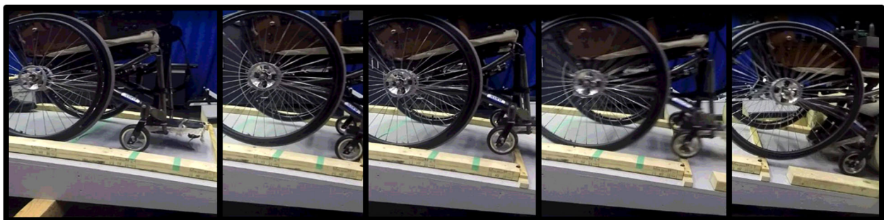
Fig. 5 Experimental sequence of events for wheelchair rolling over a high bump (3.18 cm) at 2.59 km/h.(1) wheelchair released to roll down slope, (2) casters impact bump and rear wheels lift, (3) the rear wheels return to the ground, but the momentum causes the casters to lift, (4) casters clear bump, (5) the rear wheels follow, also clearing the bump
