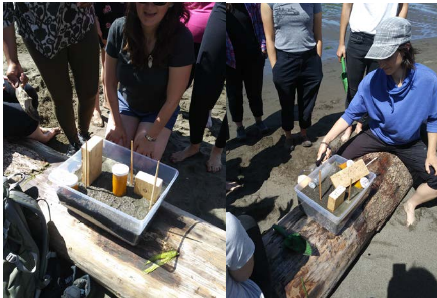
Figure 3.3.7 Before (left) and after (right) the simulation of an earthquake. The impact of liquefaction is obvious.
