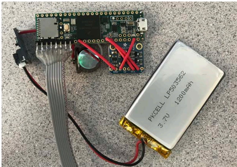
Figure 2 - Top view of electronics case completed assembly
