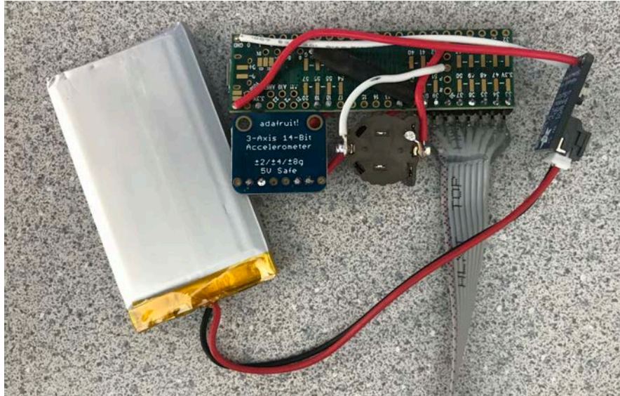
Figure 3 - Bottom view of electronics case completed assembly. Note the resistor is in the black heat shrink wrap to prevent accidental contact with other components
