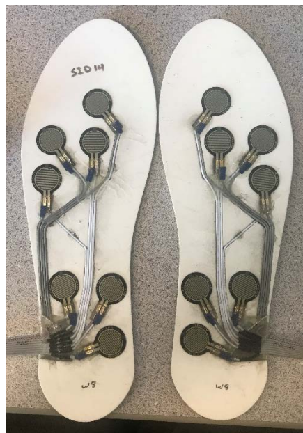
Figure 13 - A pair of insoles with FSRs and connection wires installed. Wires are all inlaid into the white foam to provide a flat top surface. The black puff foam cover has not yet been added.
