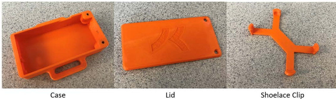
Figure 4 - 3D Printed case components
