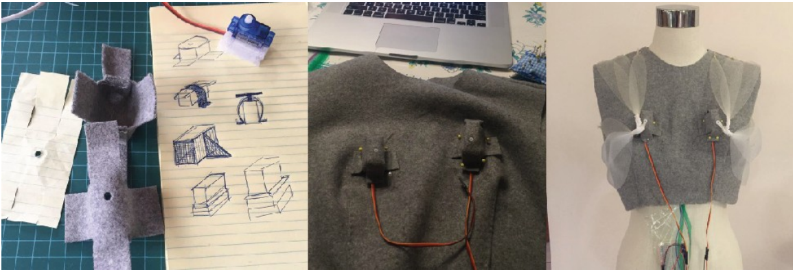
Figure 6.12. Design process of rotational motor housing.
