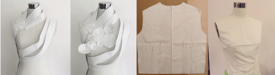
Figure 6.11. Paper draping and pattern creation for base layer
