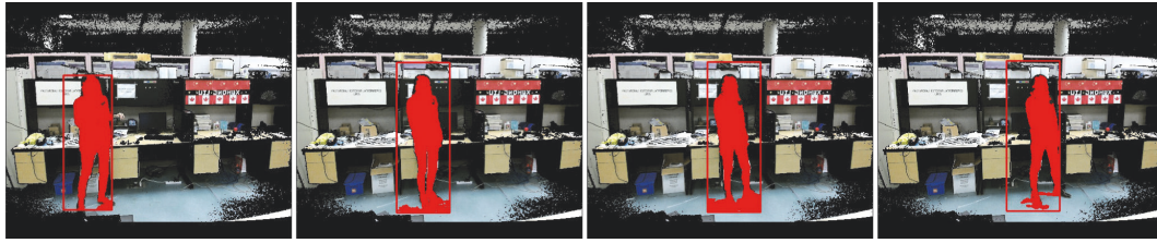
FIGURE 2: An example sequence associated with two-stage depth segmentation, that is, background subtraction and DFS in order to find the largest connected component.
