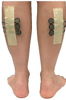
Figure 3-31 Array of three circular FSRs ® placed on human calves
