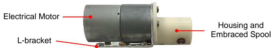
Figure 3-6 Configuration of mounted spool and housing to electrical motor
