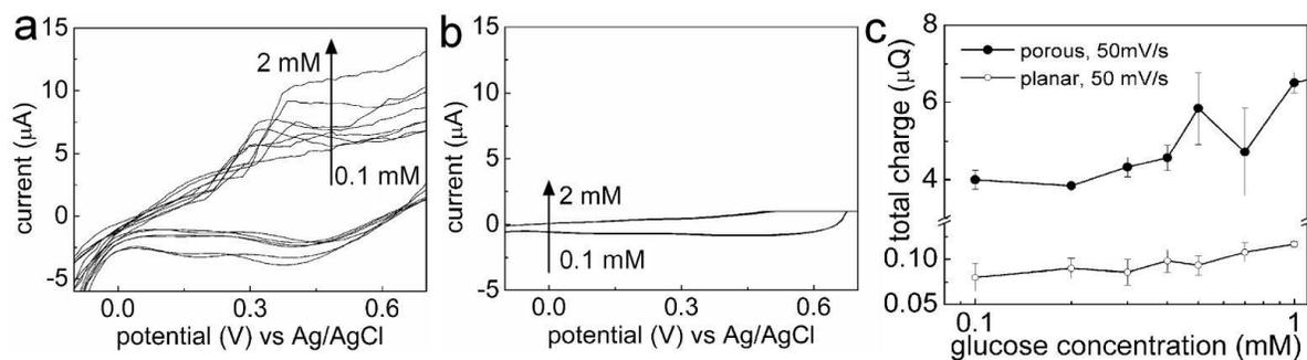
Figure 4. (a) CV scans performed at 50 mV/s with GOx coated ordered porous gold electrodes for the analysis of glucose concentrations from 0.1 mM to 2 mM. (b) CV scans of a planar gold electrode decorated with GOx also acquired at 50 mV/s. (c) Total charge generated by each electrode in (a) and (b) at different glucose concentrations.
