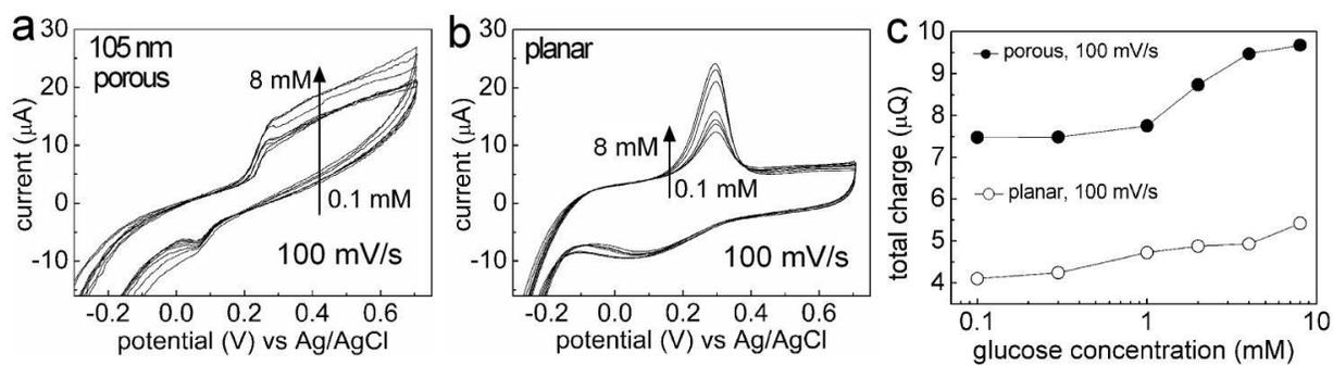
Figure 3. (a) CV scans performed at 100 mV/s with GOx coated ordered porous gold electrodes for detecting glucose concentrations from 0.1 to 8 mM. (b) CV scans of a planar gold electrode coated with GOx for the detection of glucose while scanned at 100 mV/s. (c) Total charge accumulated by each electrode in (a) and (b) during glucose oxidation over a range of glucose concentrations.
