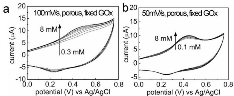
Figure 2. (a) CV scans performed at 100 mV/s with glutaraldehyde (GA) fixed glucose oxidase (GOx) ordered porous gold electrodes (105-nm diameter pores) for detecting glucose concentrations from 0.3 to 8 mM. (b) CV scans of the same electrode in (a), with CV performed at 50 mV/s.
