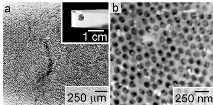
Figure 1. (a) Low magnification scanning electron microscopy (SEM) of porous (105-nm diameter pore size) gold electrode; inset: optical image of a round ( $0.071\text{cm}^2$ ) porous gold film prepared on top of gold coated silicon substrate. (b) High magnification SEM of the porous gold film with 105-nm diameter pores.
