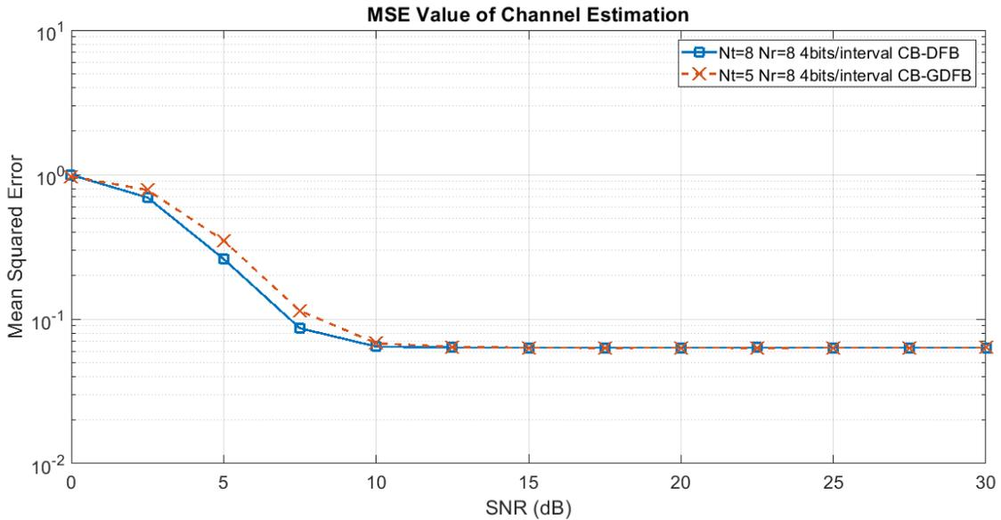
**Fig. 4.4: Mean Squared Error comparisons of channel estimation between CB-DFB and CB-GDFB for a throughput of 4 bits/interval**
