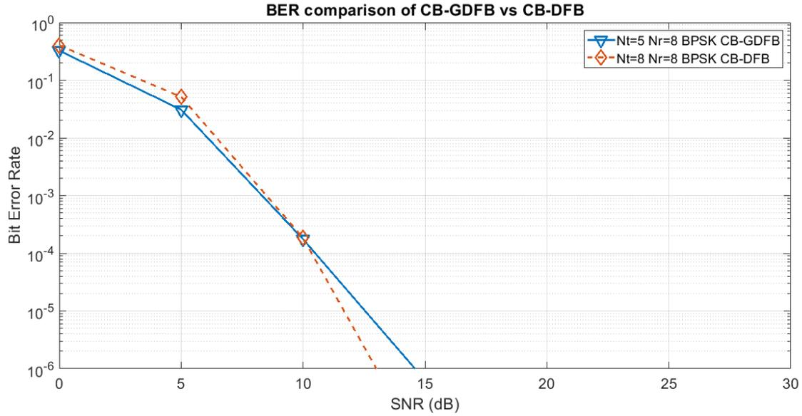
**Fig. 4.8:** BER comparison between CB-DFB and CB-GDFB at 4bits/interval. CB-DFB requires  $N_t = 8$  whereas CB-GDFB requires  $N_t = 5$  transmit antennas to achieve the same throughput.
