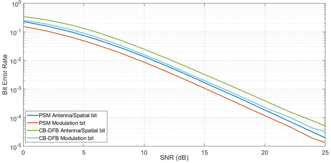
**Fig. 3.12:** BER comparison among pilot-aided spatial modulation, clustering based decision feedback coherent detection for a  $N_t = 2, N_r = 2$  system with BPSK modulation.
