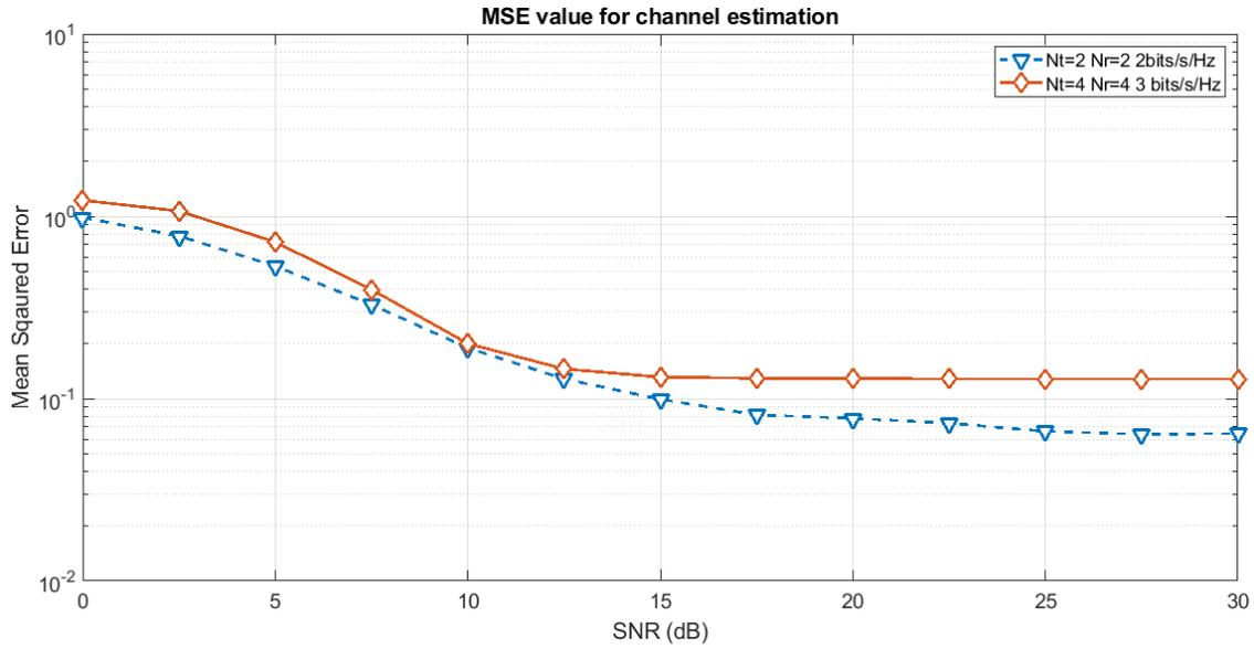
**Fig. 3.2:** Mean Squared Error Comparisons of channel estimation for  $N_t = 2, N_r = 2$  vs  $N_t = 4, N_r = 4$  CB-DFB system models
