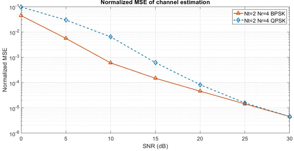
**Fig. 3.5: Normalized MSE comparisons of channel estimation for  $N_t = 2, N_r = 4$  CB-DFB systems with different modulations.**
