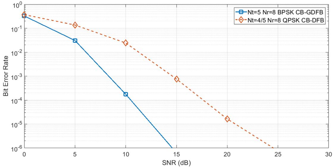
**Fig. 4.7:** BER performance of CB-GDFB Scheme versus CB-DFB Scheme at 4 bits/interval. CB-GDFB requires BPSK whereas CB-DFB requires QPSK to achieve the same throughput as of CB-GDFB.
