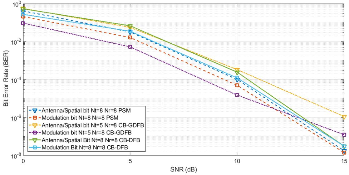
**Fig. 4.10: BER comparison among conventional PSM, CB-DFB and CB-GDFB at 4 bits/interval**
