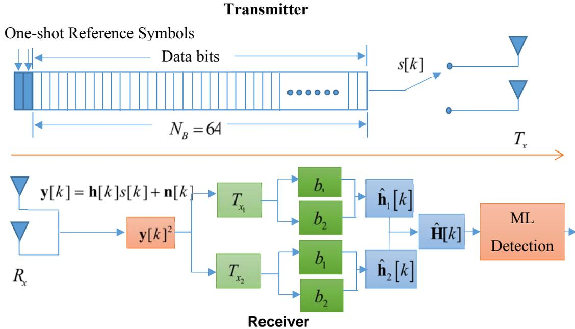
**Fig. 3.1: CB-DFB SM system model with  $N_t = 2$  and BPSK modulation**
