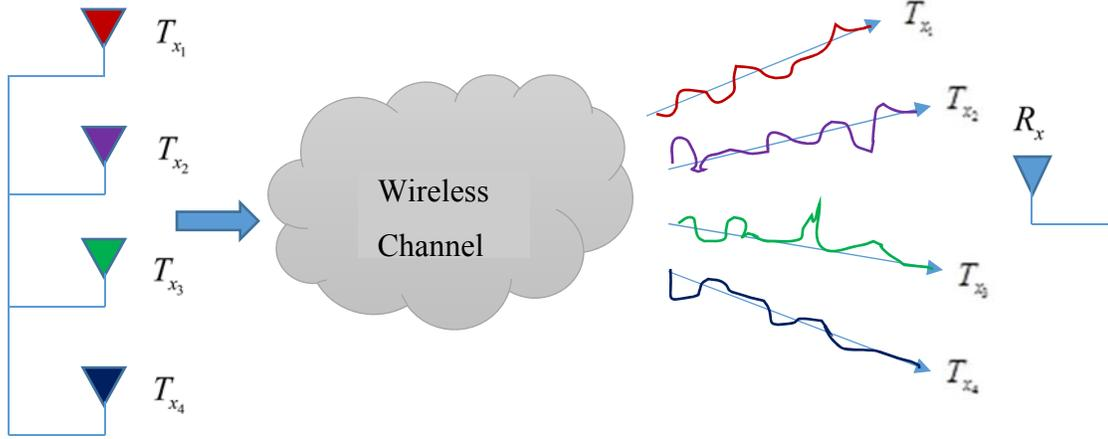
**Fig. 2.1: Spatial Modulation communication channels for a 4x1 system model**
