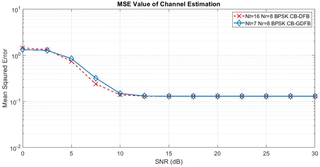
**Fig. 4.2: Mean Squared Error Comparisons for CB-DFB vs CB-GDFB for the same throughput of 5 bits/interval at different antenna configurations**
