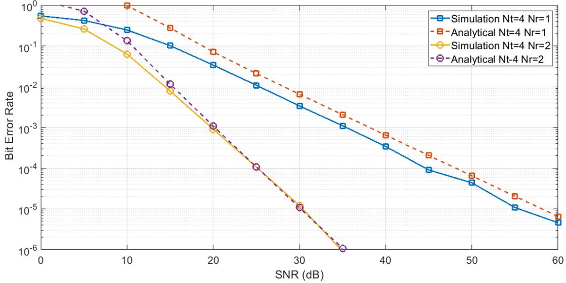
**Fig. 3.7:** BER comparison of analytical bound vs Simulation result of CB-DFB schemes with  $N_t = 4, N_r = 1$  and  $N_t = 4, N_r = 2$ .
