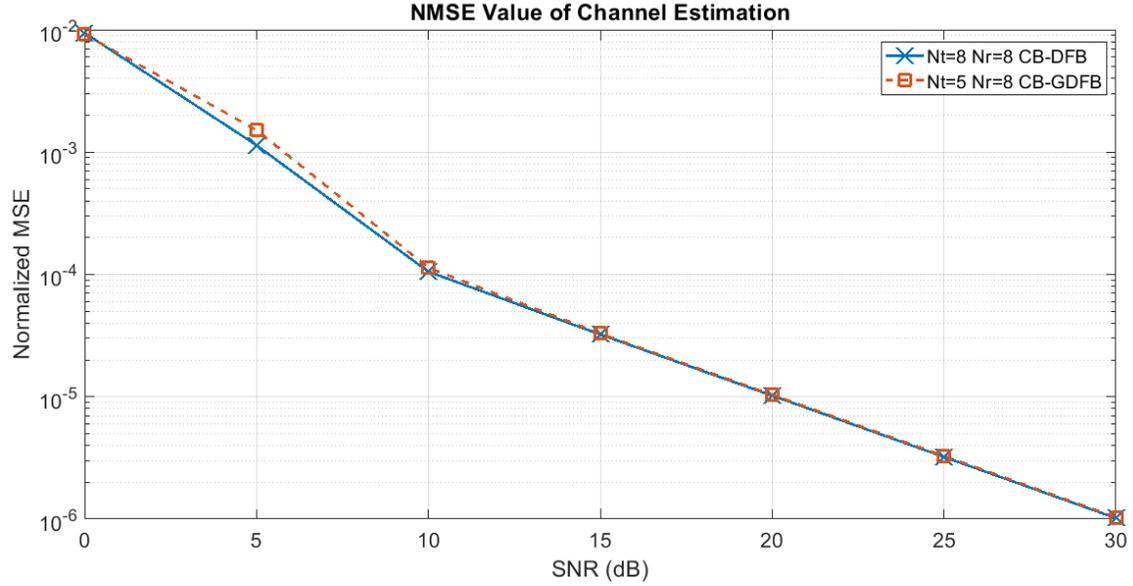
**Fig. 4.5:** Normalized MSE value comparison of channel estimation between CB-DFB and CB-GDFB for a throughput of 4 bits/interval
