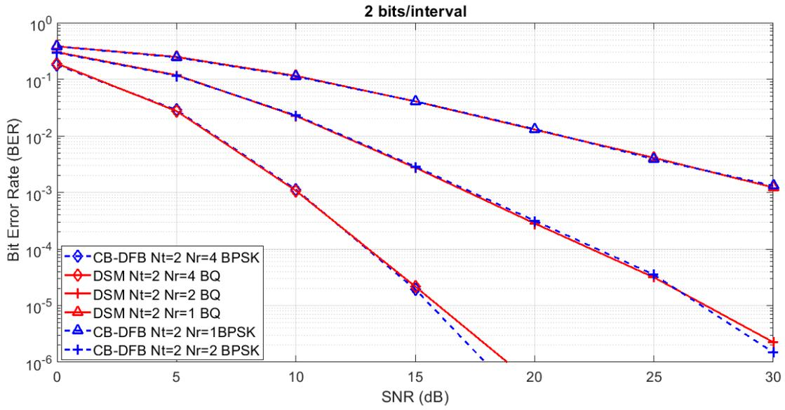
**Fig. 3.8:** BER performance of decision feedback scheme versus differential spatial modulation at 2 bits/interval transmission rate with  $N_t = 2$ . CB-DFB uses BPSK whereas DSM uses BPSK and QPSK for the two time instants respectively
