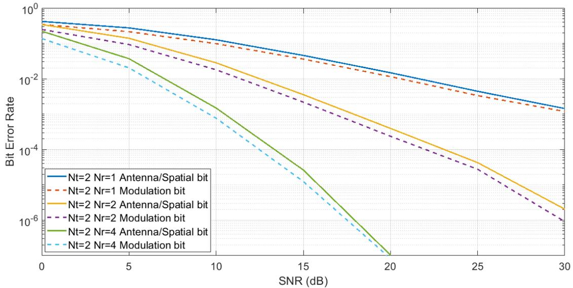
**Fig. 3.9: BER performance of spatial bits and modulation bits detection shown separately for the CB-DFB scheme with  $N_t = 2$  and BPSK modulation**
