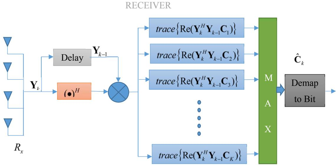
**Fig. 2.3: Receiver diagram of DSM model**
