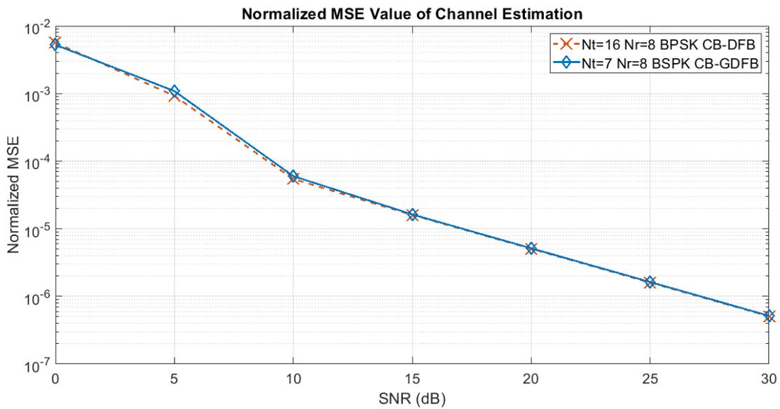
**Fig. 4.3: Normalized MSE value comparison of CB-DFB vs CB-GDFB with different antenna configurations with throughput of 5 bits/interval**
