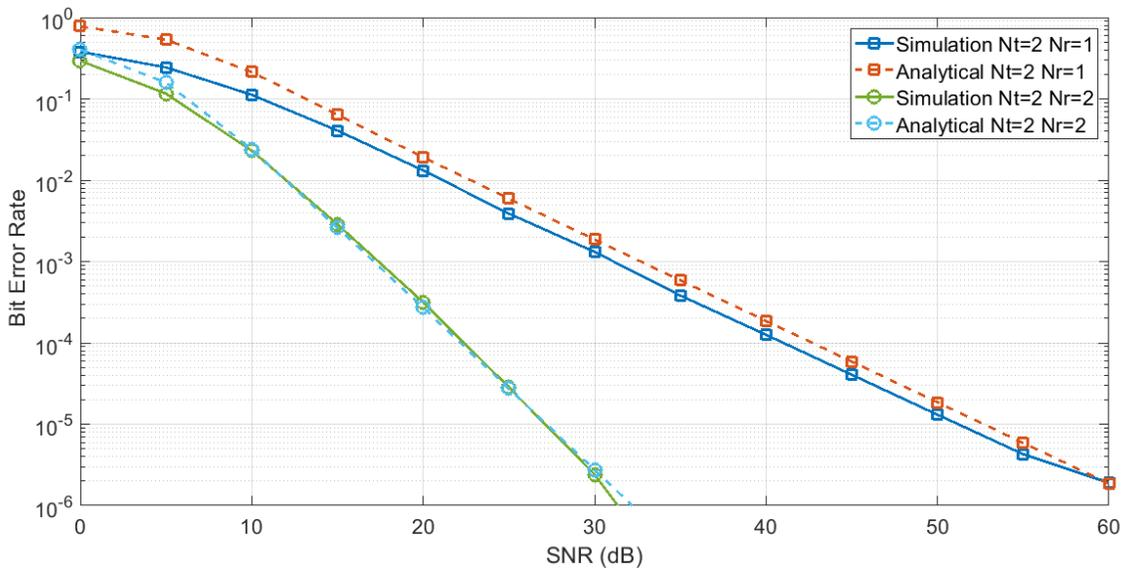
**Fig. 3.6:** BER comparison of analytical bound vs simulation result for CB-DFB schemes with  $N_t = 2, N_r = 1$  and  $N_t = 2, N_r = 2$ .
