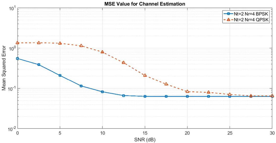
**Fig. 3.4:** Mean Squared Error comparisons of channel estimation for  $N_t = 2$  and  $N_r = 4$ , BPSK vs QPSK CB-DFB systems
