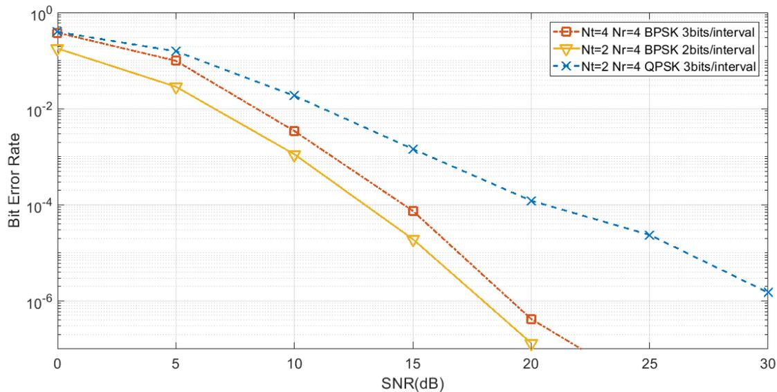
**Fig. 4.6: BER performance comparison between CB-DFB schemes for different modulation orders and different throughput**
