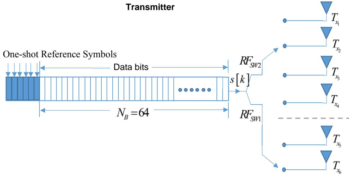
**Fig. 4.1:** Clustering based generalized decision feedback scheme with single-RF chain, two RF switches and  $N_t = 6$  transmit antennas
