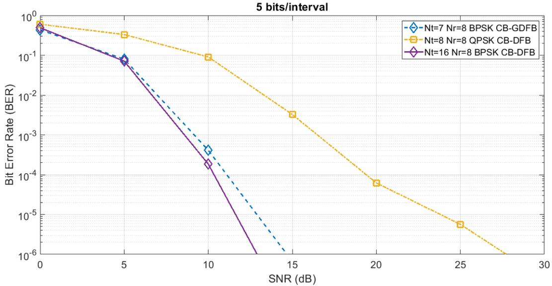
**Fig. 4.9:** BER comparison between CB-DFB and CB-GDFB at 5 bits/interval. CB-DFB requires  $N_t = 16$  initial reference symbols whereas CB-GDFB requires only  $N_t = 7$  initial reference symbols to achieve the same throughput for the same modulation constellation.
