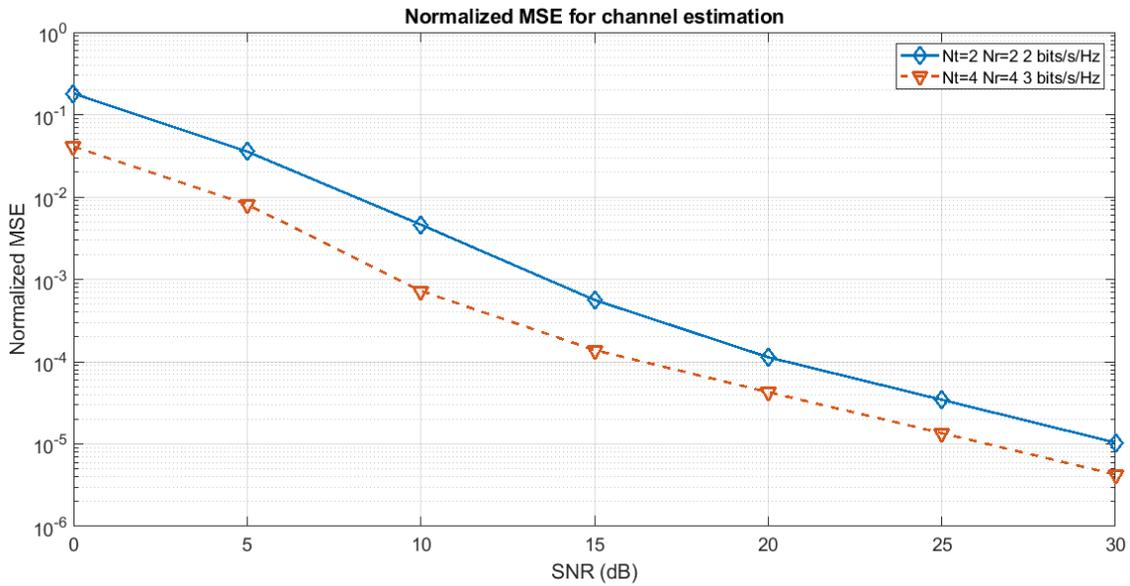
**Fig. 3.3:** Normalized MSE comparisons of channel estimation for  $N_t = 2, N_r = 2$  and  $N_t = 4, N_r = 4$  CB-DFB system models.
