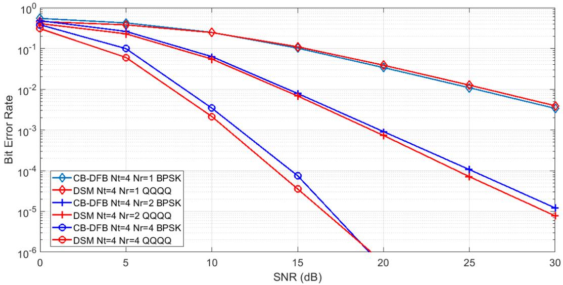
**Fig. 3.10:** BER performance of clustering based decision feedback scheme versus differential spatial modulation at 3 bits/interval transmission rate with  $N_t = 4$ . CB-DFB uses BPSK whereas DSM uses QPSK for the four time instants
