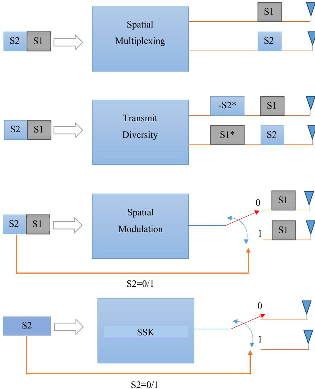
**Fig. 1.1:** Illustration of MIMO concepts: Spatial Multiplexing, Transmit Diversity, Spatial Modulation (SM), and Space Shift Keying (SSK)
