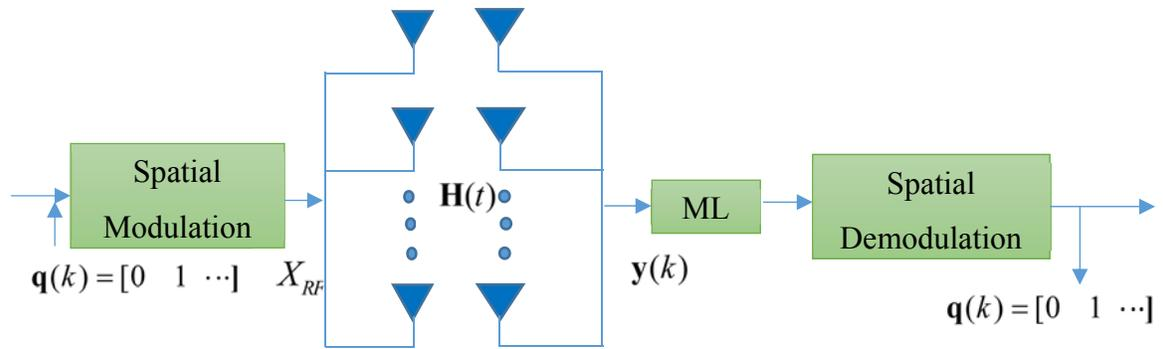
**Fig. 2.2: Simplified Spatial Modulation System Model**
