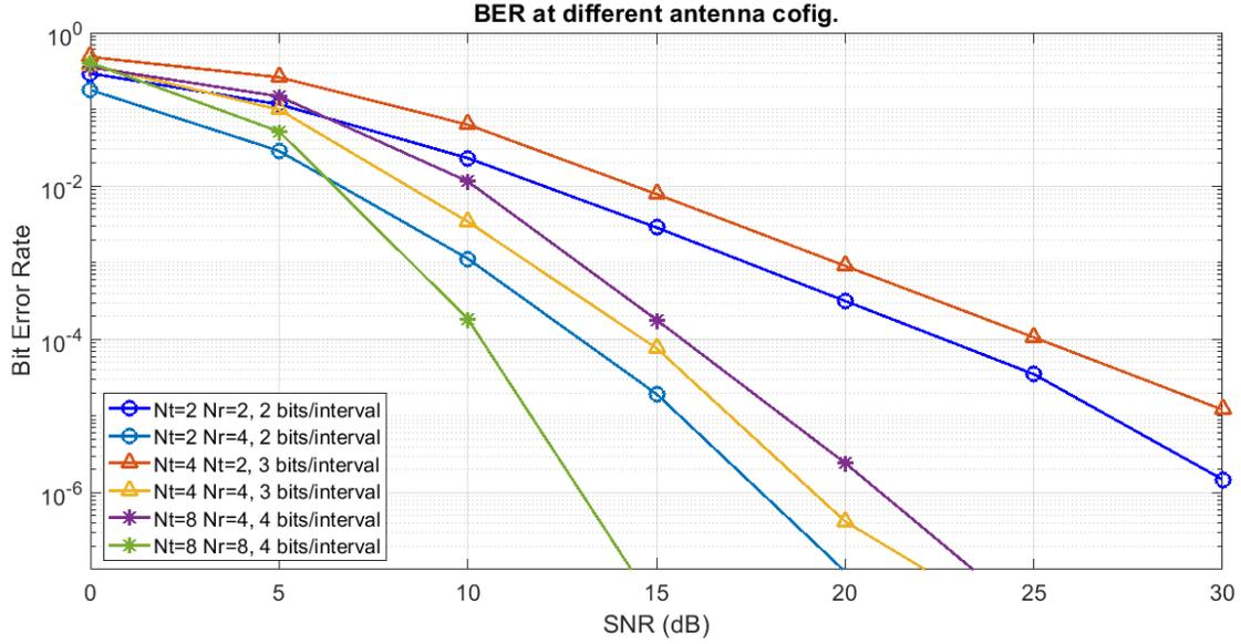
**Fig. 3.11: BER comparison of CB-DFB scheme for different antenna configurations at different throughput**
