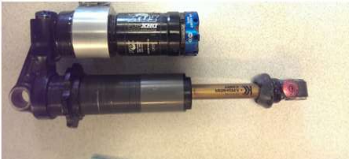
Figure 5.6 Assembled Zebra valve damper filled with MRF 140CG.
