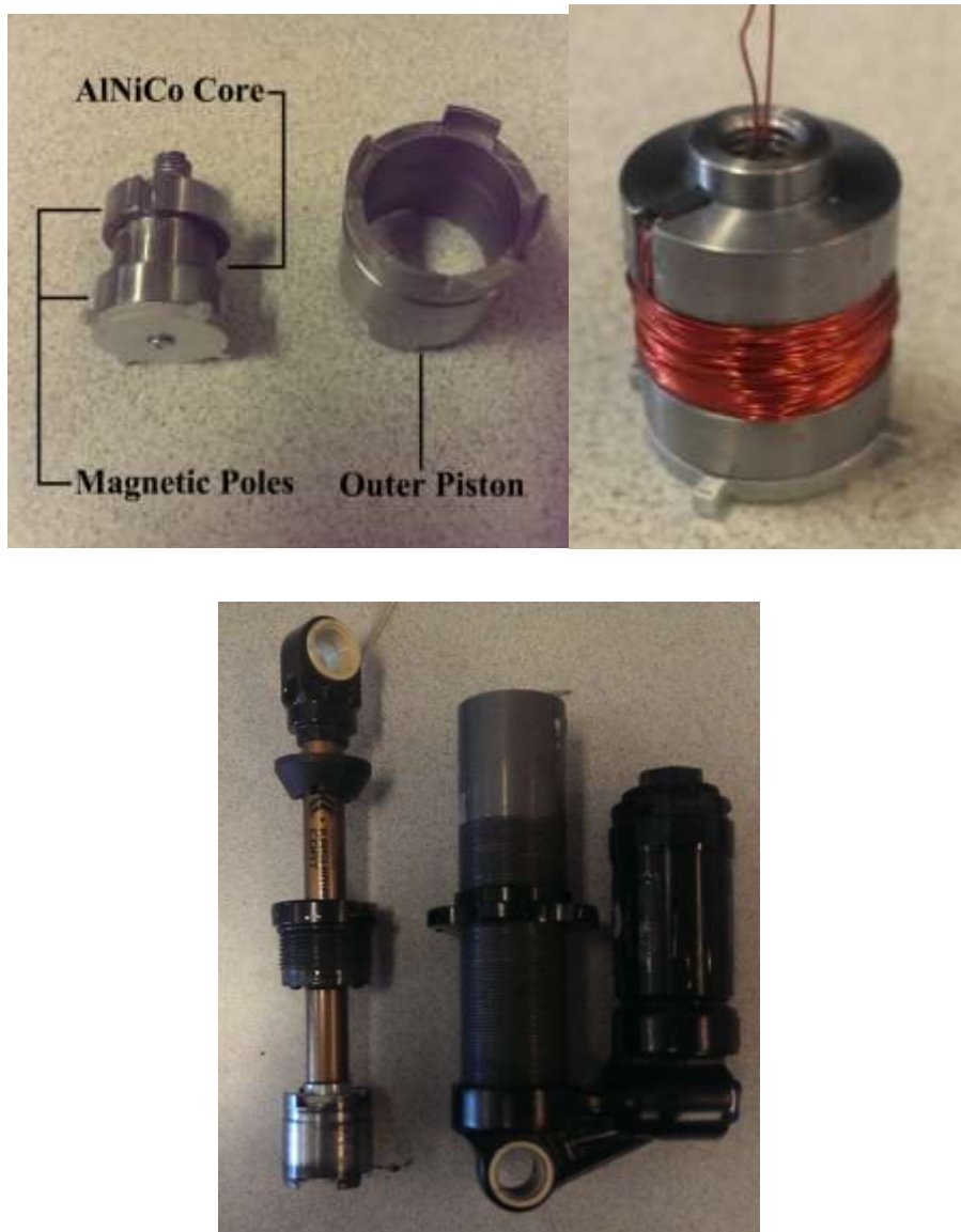
Figure 3.4 Fabricated MR damper parts based on the optimal design approach.
