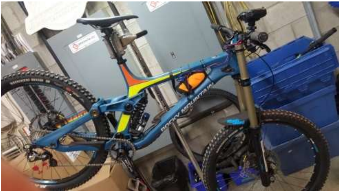
Figure 5.14 The Zebra valve damper installed on a commercial Maiden bike with battery, electronics and user interface included.
