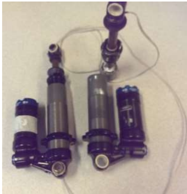
Figure 4.5 Designed prototypes of the Zebra and I-piston concept.
