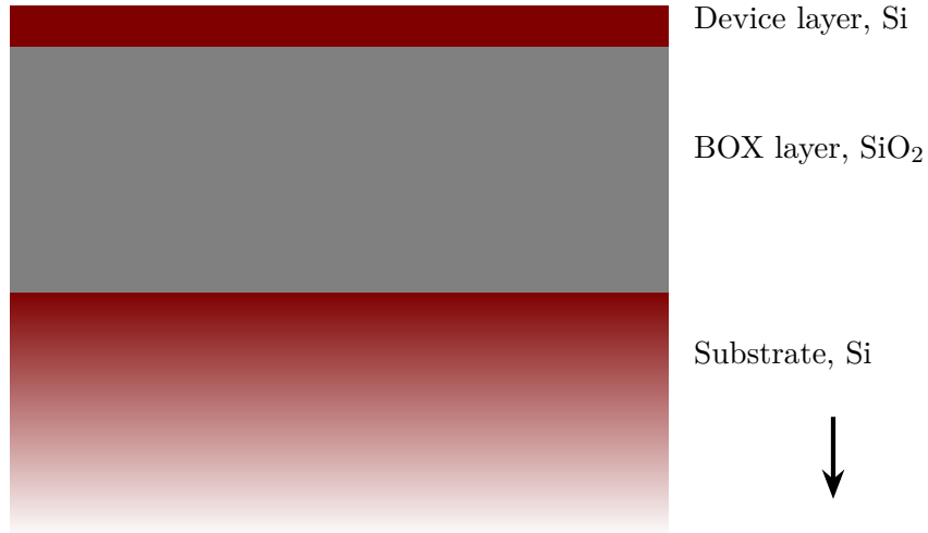
Figure 2.1: Silicon-on-insulator (SOI) substrate with silicon (Si) device layer ( \approx 100\text{--}500 nm), silica ( \text{SiO}_2 ) buried-oxide (BOX) layer ( \approx 1\text{--}3\ \mu\text{m} ), and silicon substrate ( > 500\ \mu\text{m} ).
