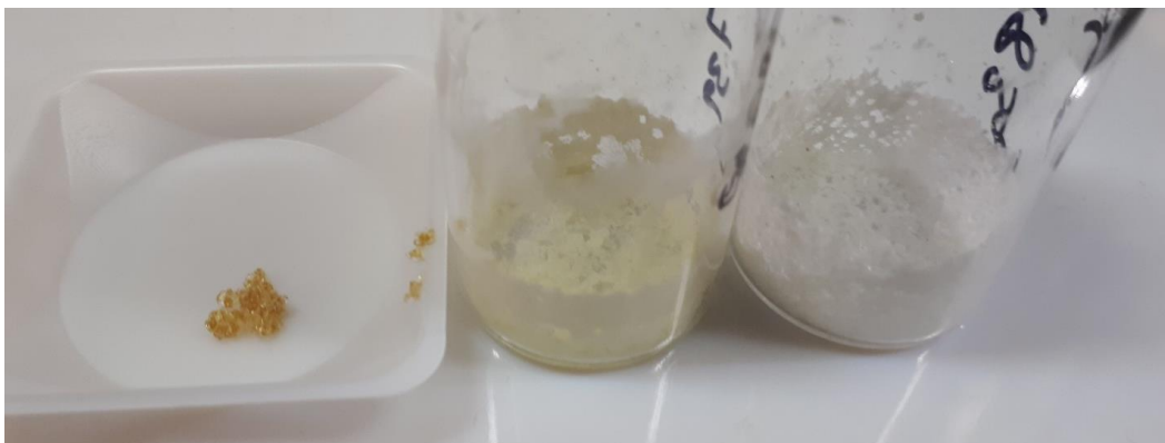
Figure 3.1 Visual Purity of Thiopyranone: (L-R) Commercially available, Purified with just Charcoal, Purified with Charcoal and Silica Plug.
