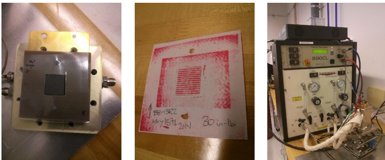
Figure 2.1: Setup of a fuel cell including: a.) a gasketed MEA before second flow field, current collector, and hardware addition + compression; b.) pressure paper demonstrating sufficient compression of the GDLs (dark lines following flow fields ridges but not connecting); c.) resultant fuel cell in operation on the fuel cell test station.
