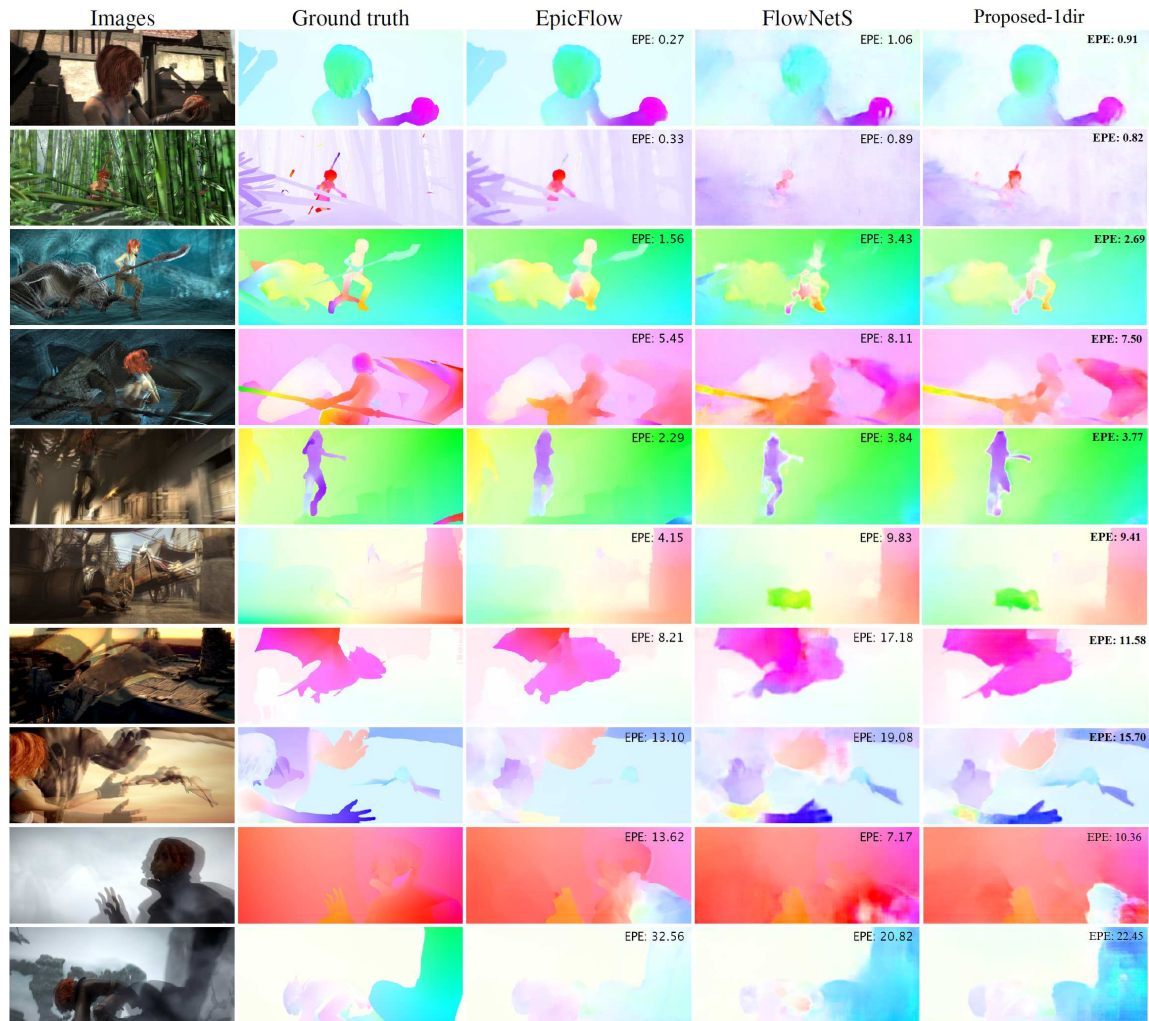
Figure 6.7: Predicted optical flows on the Sintel Final dataset. In each row from left to right: overlaid image pair, ground truth flow, the predicted results of EpicFlow [74], FlowNetS [18], and Proposed-1dir RC-LSTM. Endpoint error (EPE) is shown at the top-right corner of each prediction. In most cases (Row 1-8), the proposed method produces visually better results with lower EPE than the FlowNetS. Although the EPEs of the proposed method are somewhat worse than that of EpicFlow, our model often produces better object details, see Row 3-5, 7-8, 10.
