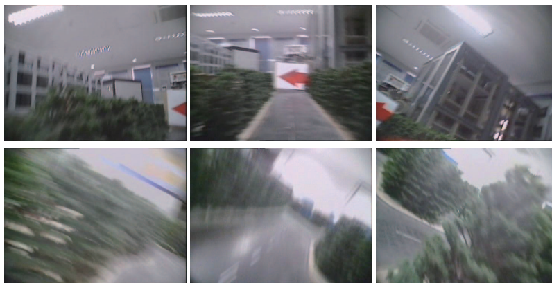
Figure 3.7: Sample video frames that our orientation network classifies correctly. The top frames contain object of interest while the bottom frames do not. The ground truth orientation label for each frame from left to right: left, middle, and right.
