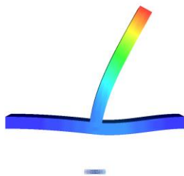
Figure 3.4. (a) Modal analysis of the T-beam microresonator simulated using Architect™. (b) The pendulum mode shape with natural frequency 1.4145 MHz. (c) The spring mode shape with natural frequency 2.8419 MHz. (blue-no displacement and red-maximum displacement)
