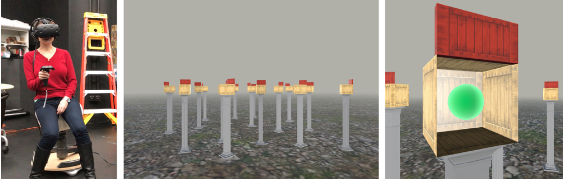
Figure 2.2: Left: Participant wearing an HMD (HTC VIVE) and sitting on the NaviChair locomotion interface. Middle: Visual stimuli of the virtual environment designed to eliminate all visual landmarks. Right: By approaching the box from its front side (the side denoted by a red banner), participants can make the box automatically open to see whether there is a ball inside, and collect the ball by touching it with the controller.
