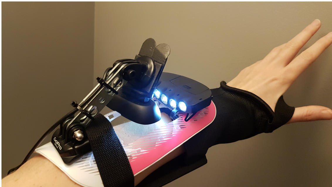
Figure 5.4: Custom made set-up of a wearable camera for recording a video of participant's skin for identifying goosebumps and shivers.
