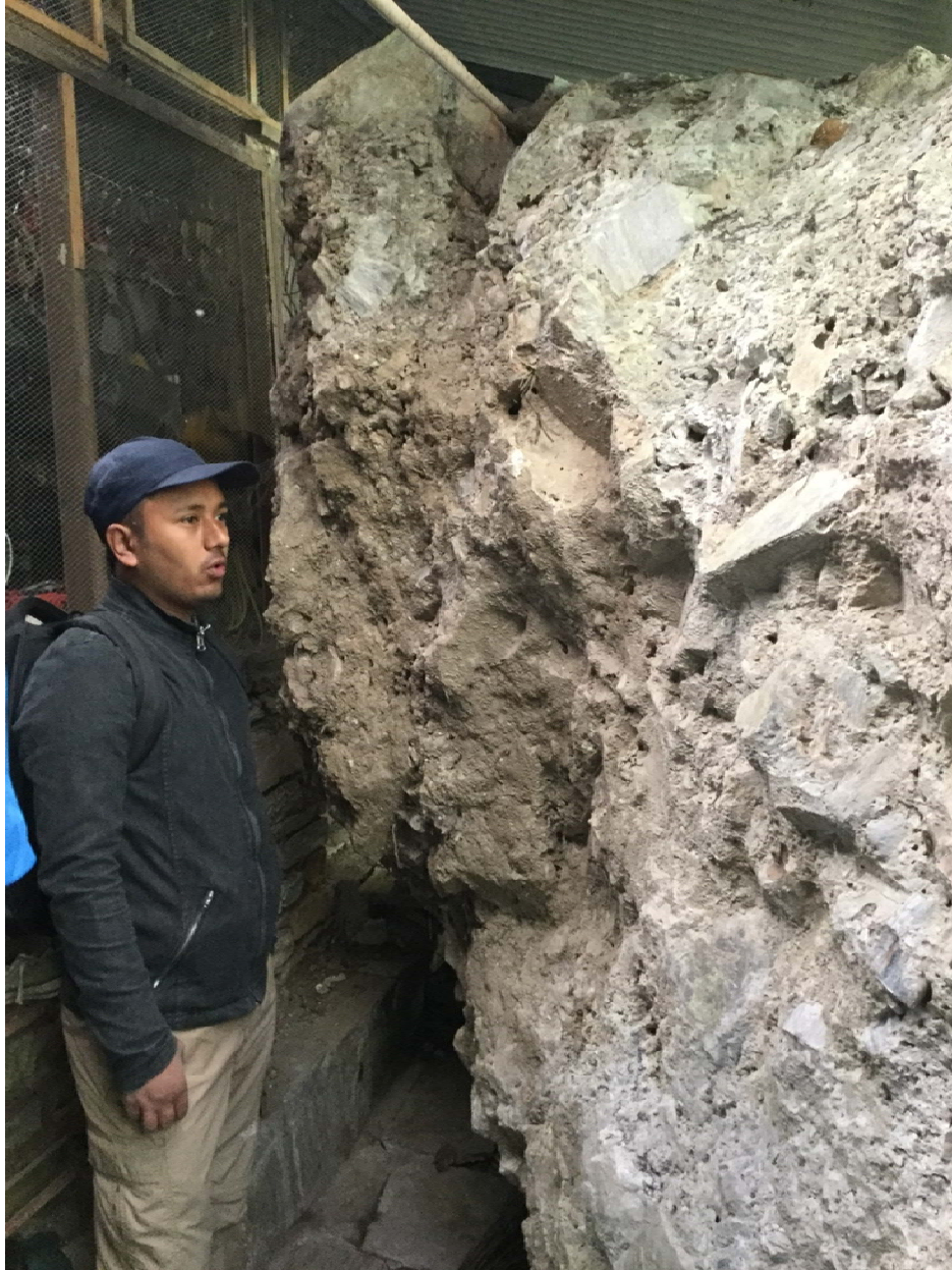
Figure H 2. Rockfall boulder with evidence of tectonic cataclasis that impacted the back of an equipment room at TLR. Photograph taken November 13, 2016.
