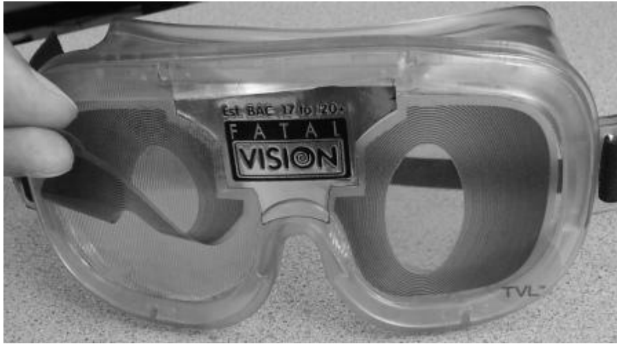
Figure 3.3. Silver Label Fatal Vision goggles which equal to BAC of 0.17 to 0.20 and tunnel vision lenses attached to them
