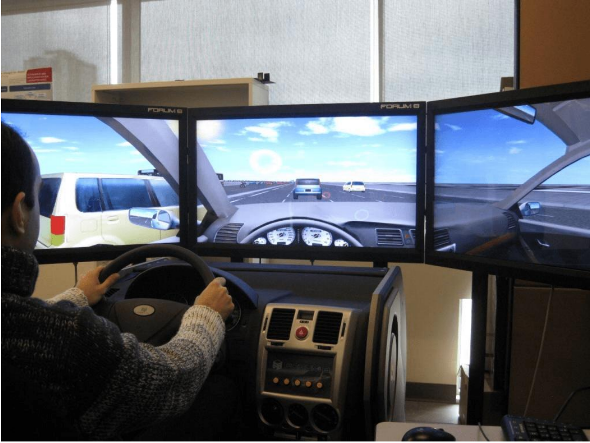
Figure 3.1. Driving simulator used for data collection
