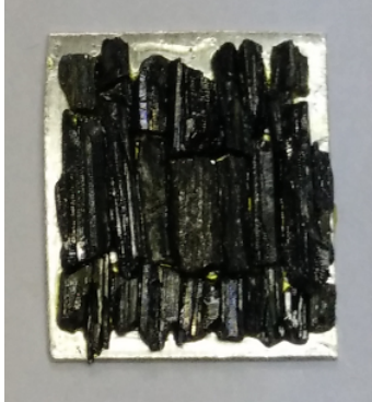
Figure 2.6: The oriented mosaic of CePtPb single crystals on a silver plate used in the \mu SR experiment.
