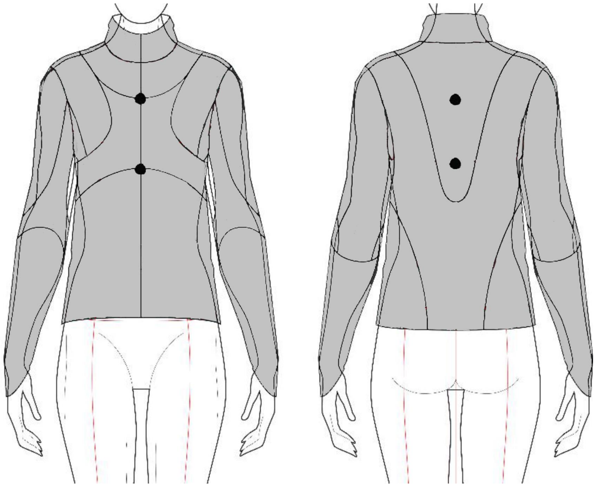
Figure 2-2 Placement of four iButtons over the base layer and under the jacket (black circles)
