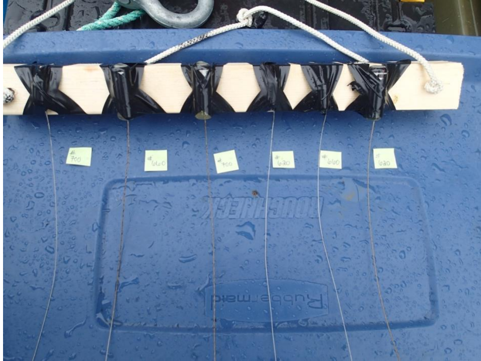
Figure 2. Tag set up for radiotelemetry tags for drift detection probability testing. Gastric and external tags were fixed to a wooden block and towed at 1 meter depth behind the boat for a known amount of time. n = 6
