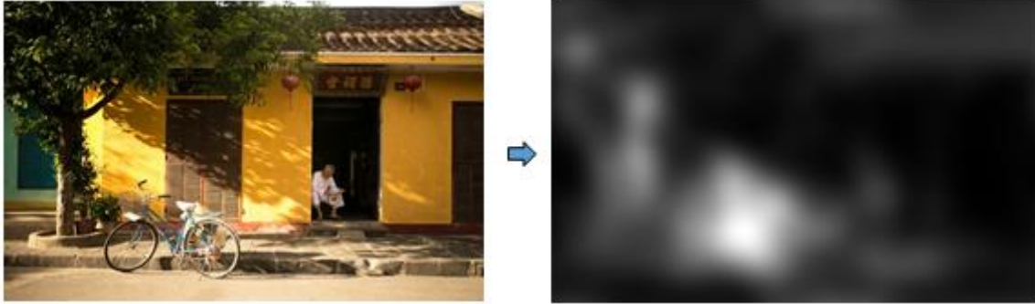
Figure 8: Input image I(x, y) (left) and its AWS saliency map S(x, y) (right)
