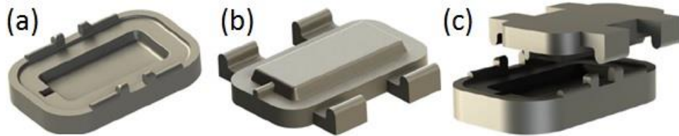
Figure 9 - Bottom (a) and top (b) half of the old mold, and the mold assembly c).
